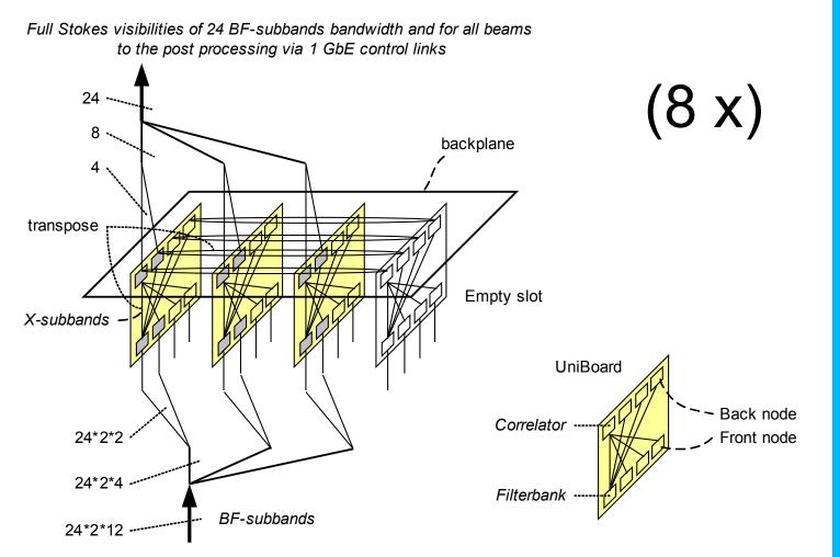
All beams with each 24 dual pol BF-subbands from 12 telescopes
