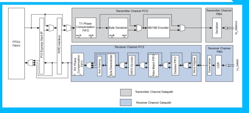
Reduce the number of interfaces by combining multiple low speed interfaces into a single high-speed interface SerDes included inside FPGA with signal conditioning
